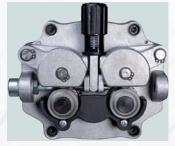
Simple, but sturdy, wire drive assembly. Solid aluminium components with drive rollers top and bottom.
